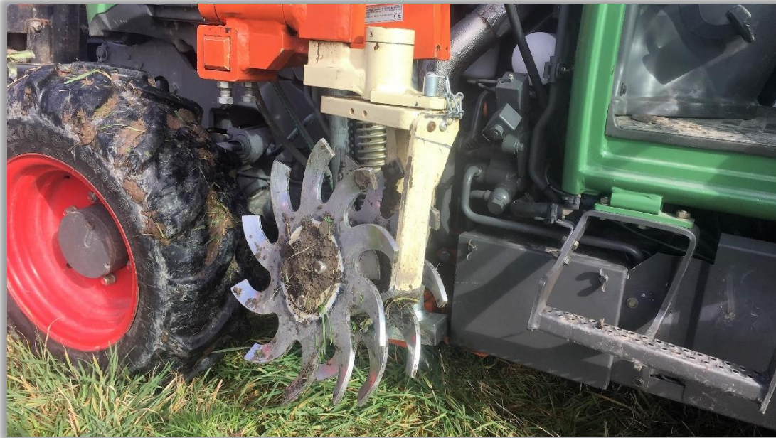
FIGURE 5. BRAUN ROLLHARKE FOR ROUGHING UP THE UNDER-VINE STRIP PRIOR TO MULCH APPLICATION. BETTER FACILITATE MULCH AND SOIL INTERACTION.
