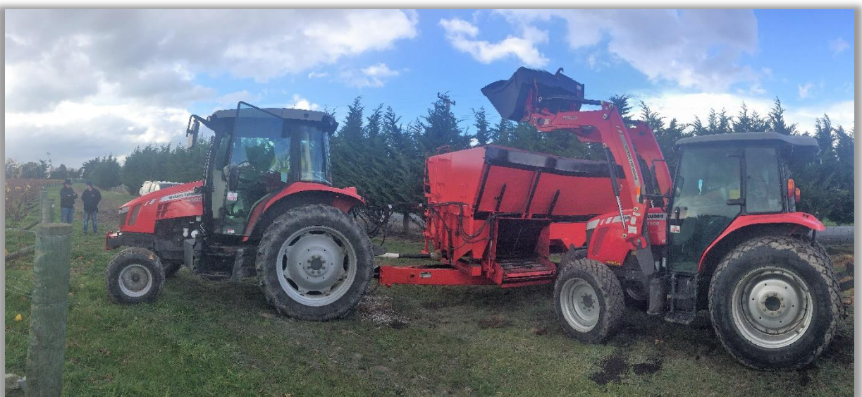
FIGURE 1. SIDE DISCHARGE HOPPER FOR SPREADING MARC MIX UNDER VINE. PHOTO LIBRARY. MCMILLAN (2019).
